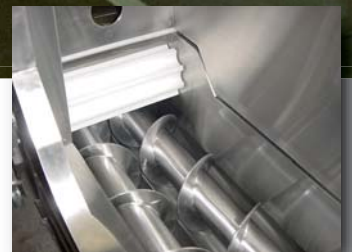
Sanitary Stainless Steel Augers work the butter prior to pumping
